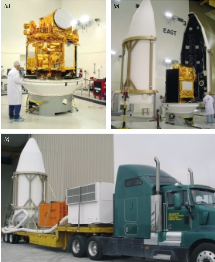
Figure 2: (a) The completed ROCSAT-2 satellite with its telescope mounted on top of the main body of the satellite - undergoing tests. (b) The ROCSAT-2 satellite about to be enclosed in its protective fairing prior to launch. (c) ROCSAT-2, now in its fairing, about to be transported to the launch pad at Vandenberg Air Force Base (AFB) in California. (Source: National Cheng Kung University)
