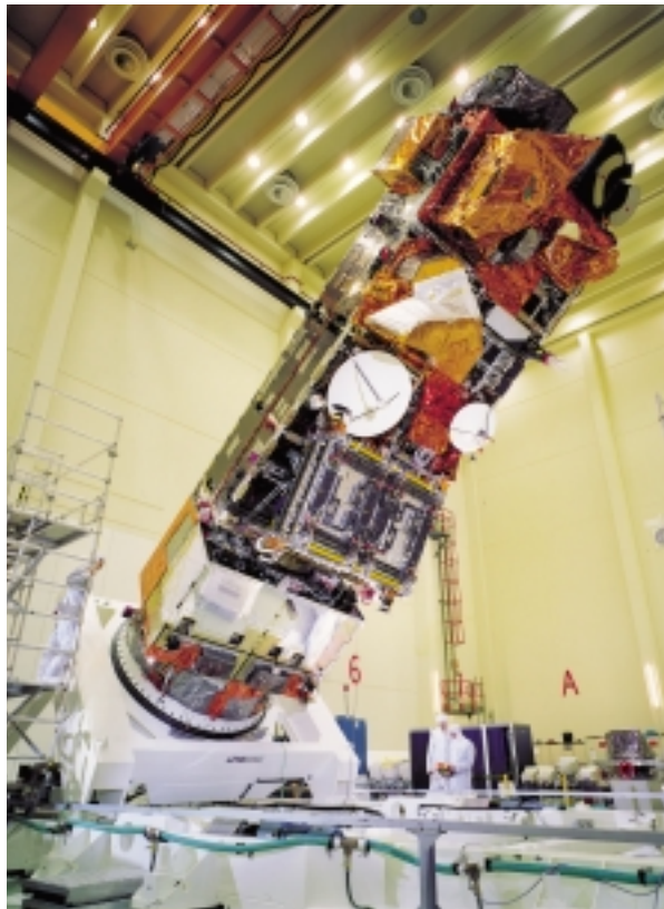
Envisat under test. (Source: ESA)
