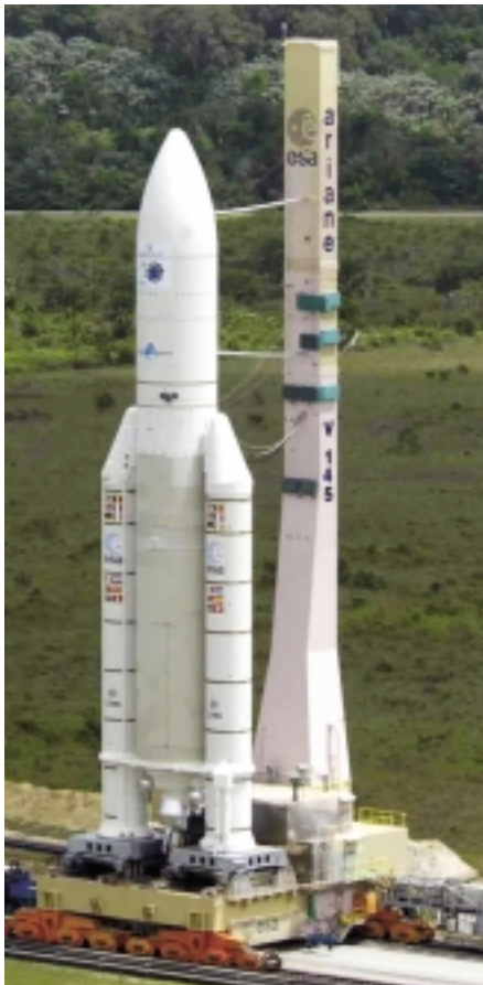
The roll-out of the Ariane-5 launcher from the Final Assembly Building at the Kourou Space Centre with Envisat mounted on top of the main rocket. (Source: ESA)
