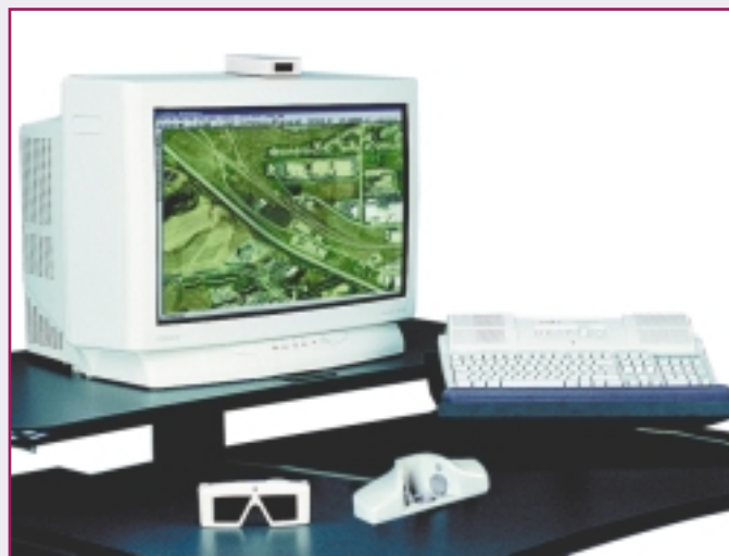
The ImageStation 2000 DPW introduced at the Conference by Z/I Imaging. This redesigned and upgraded version of the ImageStation series features a special support table with electrically adjustable height control of the digitizing and monitor surfaces. The PC with its twin 866 MHz Intel Pentium III processors and its storage drives and electronics is accommodated in a special rack enclosure located underneath the table. (Courtesy Z/I Imaging)
