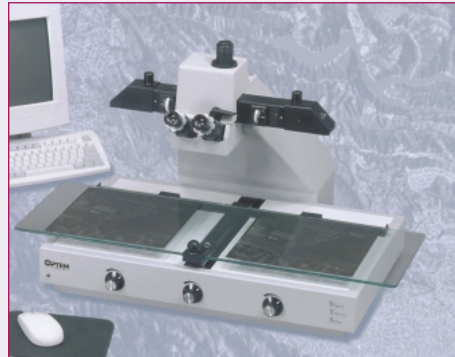
The Optem Digital Transfer Scope (DTS) allows the viewing and interpretation of stereo-pairs of hard copy aerial photos superimposed over the corresponding digital map data. (Courtesy Optem)
