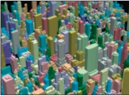
Figure 2. A perspective visualization of part of New York city. This is based on the accurate 3D terrain and building model data extracted from stereo-pairs of aerial photographs of the city by Vexcel's mapping and GIS group.
