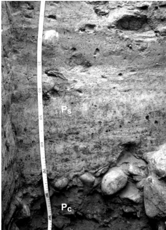
Fig. 8. Coarse-grained bar platform ( P_c ) topped by fine-grained supraplatform deposits ( P_s ) at Exit Pool (denoted by grey patch in Fig. 7h; flow from left to right). Note the occasional floating gravels and cohesive nature of the P_s .
